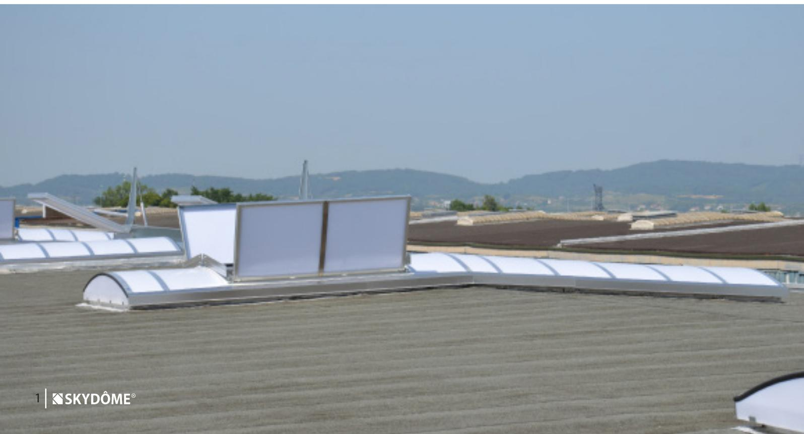
The ARCADEF® ROOF Pneumatic is fully assembled in the factory. On site, installation is greatly simplified. The device only needs to be placed and fixed on the vault. Adaptable to ARCADE vaults with a chord length of 2000 to 4000 mm, its constant radius of 2800 mm adapts to the ARCADE vault in a fast and efficient way.
