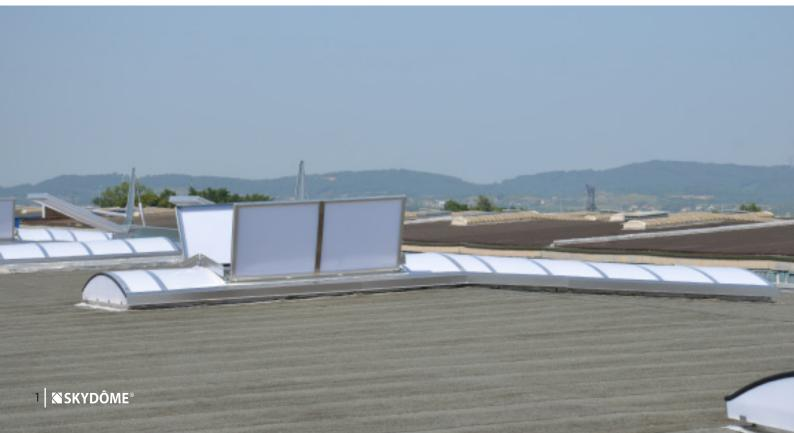
The ARCADEF<sup>®</sup> ROOF Pneumatic is fully assembled in the factory. On sote, installation is greatly simplified. The device only needs to be placed and fixed on the vault. Adaptatble to ARCADE vaults with a chord length of 2000 of 4000 mm, its constant radius of 2800 mm adapts to the ARCADE vault in a fast and efficient way.
